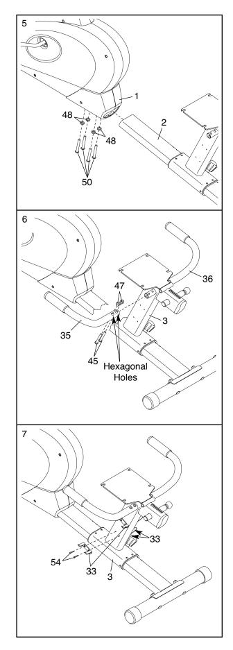
Apply a generous amount of the included grease to the Pivot Axle (40). Then, orient the Backrest Bracket (13) near the Seat Carriage (3) as shown.
